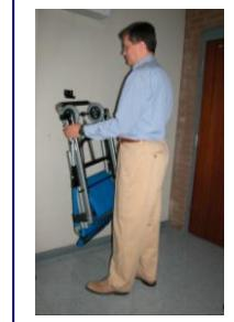
2. Place the Evacuation Chair on the floor and adjust the handle to the required height by holding the chair in place with your foot and pulling upwards on the handle. The Handle can be lowered using the release button located on the inside of handle tube.
