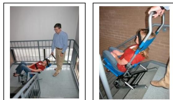
6. When the bottom of the stairs is reached, tilt the chair slightly forwards and pull the rear wheels out and away from the track so you are able to continue to safety on flat ground using all four wheels.
