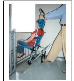
3. Push the Evacuation chair down the first step carefully until the track is sitting level on the steps; ensure you are holding the Evacuation Chair securely. T
