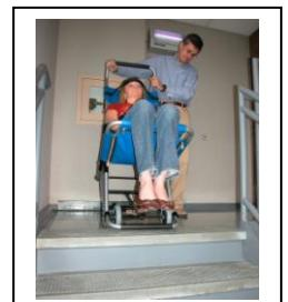
2. Tilt the chair forwards and push the rear wheels in to the folded position so the track is free to sit on the stairs without interference.
