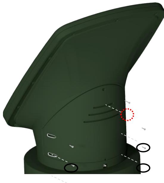
Reattach the rear hatch using the screws provided. Caution: one of the screws (marked here in RED) is 5 x 30, i.e. longer than the other 4 screws, which are 5 x 20.
