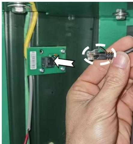
Connect the RJ9 connector to the board on the bottom of the Aivia SOLO
